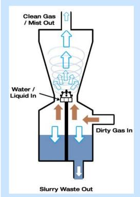
The VGS acts as a wet scrubber combined with a high-powered I.D. fan to ensure continuous a continuous flow through the Venturi chamber and exiting the flue gases to atmosphere.
